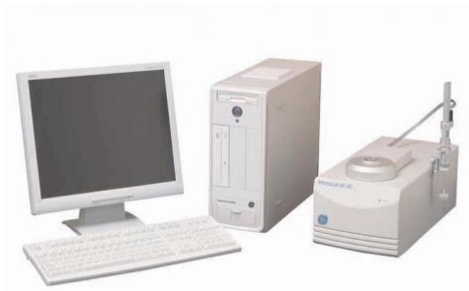
Figura 11. Microcalorimetro Microcal VP-ITC
