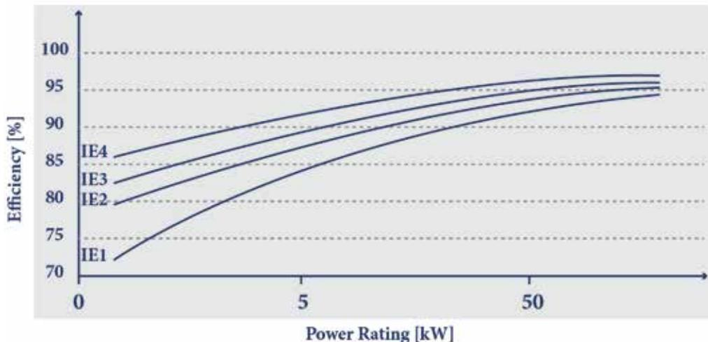
Figure 6.6 Efficiency of Electric Motors
