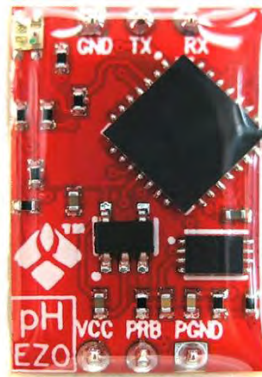
Figura 0.4 Circuito EZO pH (AtlasScientific b, 2015).
