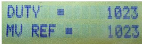
Duty Cycle Screen shows internal values for the duty cycle and motor voltage set point. This is mostly used for troubleshooting.
