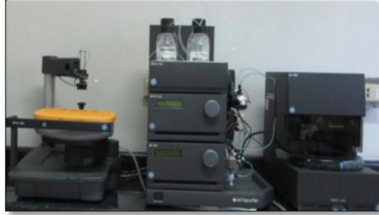
Figura 15. Cromatografo Äkta Purifier 10 UPC (GE Healthcare®), un auto-muestreador A-900 (GE Healthcare).
