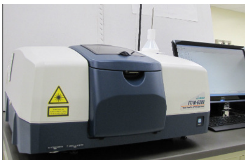
Figure 3.2 Jasco FT/IR-6300A equipment used in the work.
