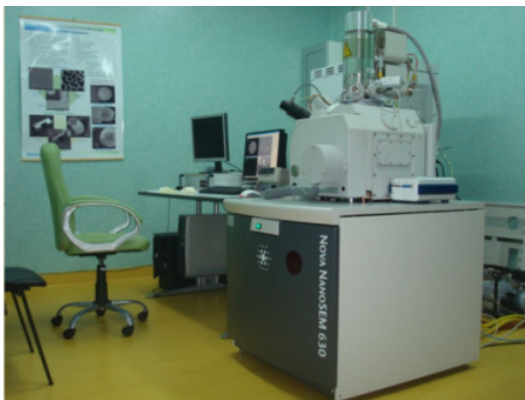
Figure 3.1 Illustration for FEI Nova NanoSEM 630, used in the work
